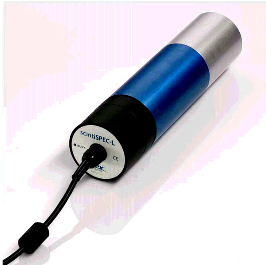
Figure 6: 2"x2" BrillanCe B380 detector with scintiSPEC-L plug-on MCA
