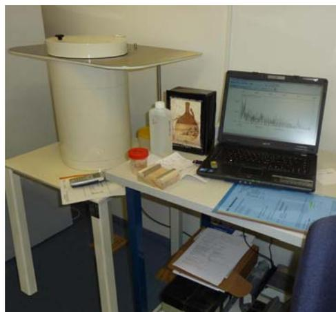
**Figure 3.** External  $\gamma$ -ray spectrometer: Lead castle with NaI(Tl) detector and MCA inside, laptop PC and printer
