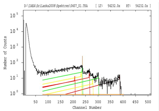
Figure 4. Analysis of an alpha spectrum taken from a sample of pitchblende powder containing  $^{238}\text{U}$  and progeny
