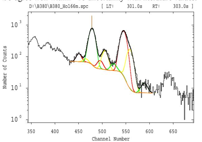
Figure 5. Final result for a region around 750 keV of a  $^{166}\text{mHo}$  spectrum which was measured with a  $2''\times 2''$  B380 detector and automatically analysed
