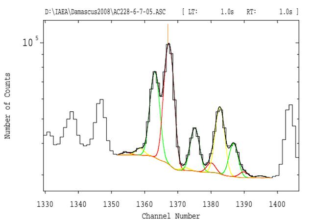
Figure 3. Fully automatic analysis of a region around 1001 keV in the  $\gamma$ -ray spectrum from a U/Th-containing source
