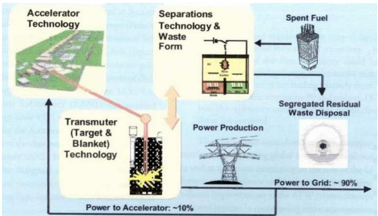
**Figure 3: Components of an ADS System**
