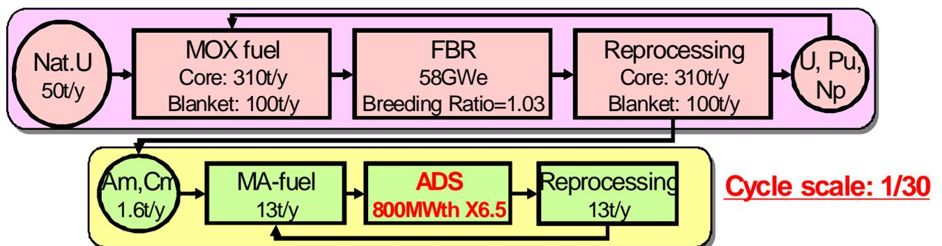
**Figure 4:** Schematic of a dual strata transmutation system. Quelle: PARTRA meeting, 2008
