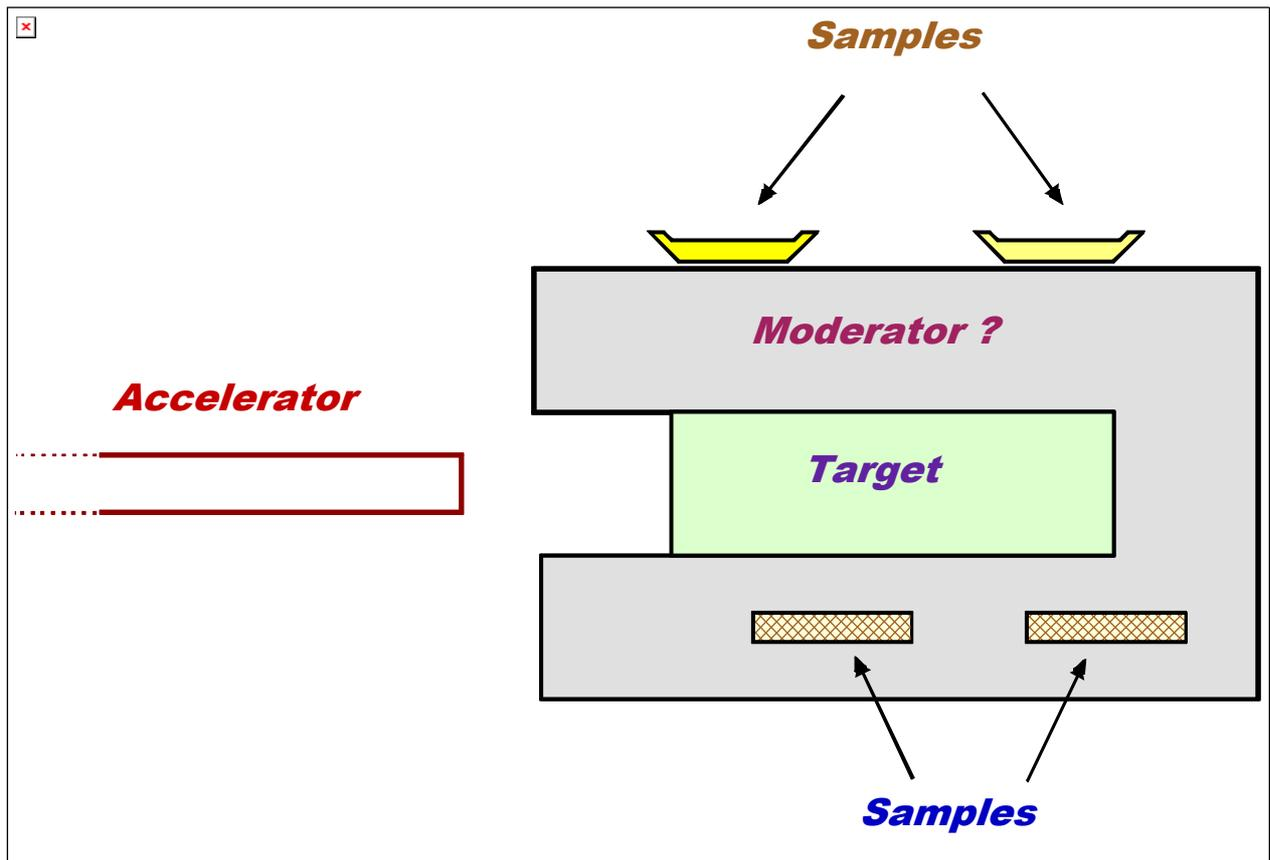
Figure 2: Schematic display of essentials in an Accelerator Driven Transmutation setup. The target may be of very complex composition and the use and nature of a neutron moderator must be investigated.
